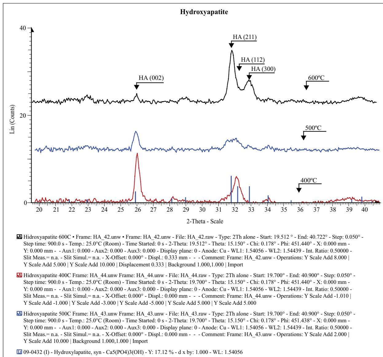
**Figure 3.** XRD of samples deposited at substrate temperatures of 400°C, 500°C and 600°C. The markers on top of the 2-Theta-Scale correspond to the peak positions and relative intensities from HA 09-0432 standard card.
