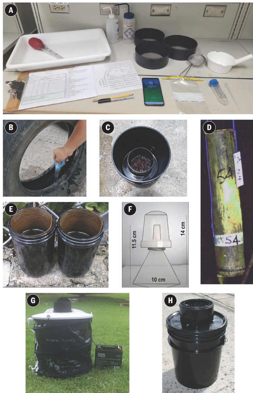
Figure 2. Tools used for surveillance of immature and adult stages of Aedes aegypti : A, equipment used to collect larvae and pupae from water-filled containers; B, water collected from a discarded tire; C, polyacrylamide (PAM) gel ovitrap; D, bamboo internode larvitrap; E, paired ovitraps; F, miniature funnel trap; G, BG-Sentinel 2 trap; and H, Autocidal Gravid Ovitraps (AGO).
