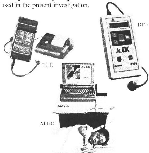
Figure 1. Three types of hearing screening devices, the Natus Algo 2, an AABR, the Otodynamics EchoCheck, a TEE, and the Bio-logic AuDx, a DPE.
